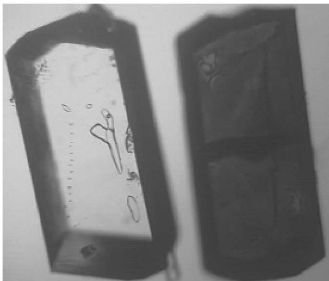
Fig. 11. Transmission light micrograph of recrystallised trehalose before (left-hand crystal) and after (right-hand crystal) exposure to DVS cycle described in text.
